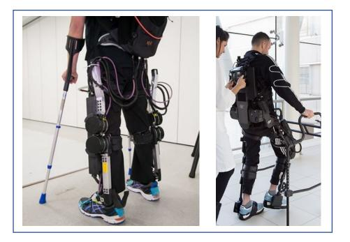
Figure 21: Exoskeletons to support gait training (Pictures: Fondazione Santa Lucia)
