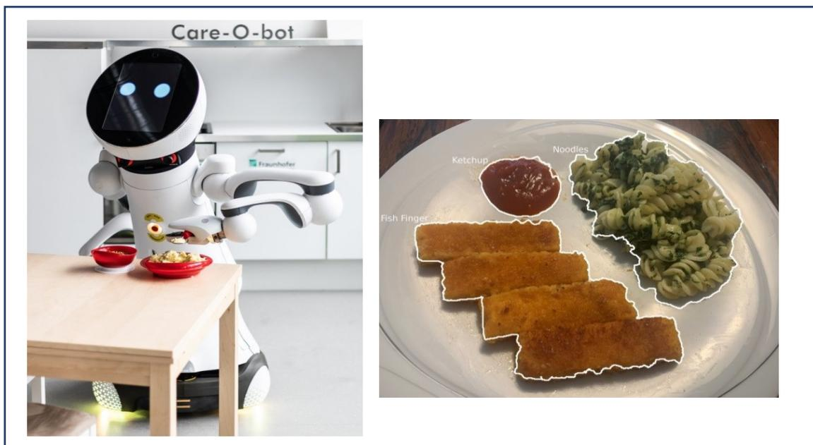
Figure 29: The Care-O-Bot 4 is able to identify food on a plate, to pick it up with a spoon and to present it in front of a person's mouth (Picture: R. Bez © Fraunhofer IPA)
