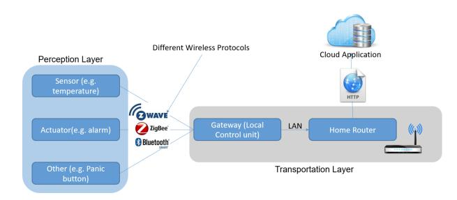
Figure 32: Common end user IoT Architecture
