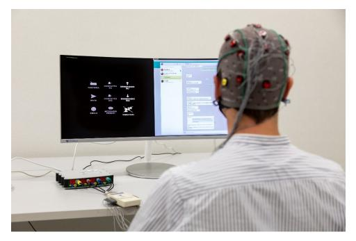
Figure 75: An example of a P300-based BCI setup
