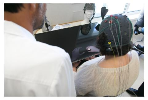
Figure 76: SMR-based BCI for upper limb rehabilitation after stroke
