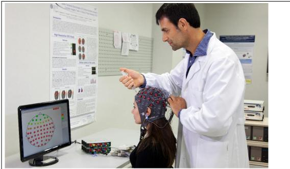
*Figure 71: The operator is putting conductive gel between the electrodes and the scalp od the user.*
