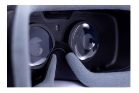
*Figure 52: absorbent foam padding in VR headsets*
