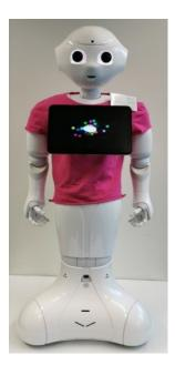
Figure 27: The interaction robot PEPPER (Softbanks) can play music, dance and recognize people. On its tablet monitor, additional functions can be added (Picture: K. Türkogullari, Frankfurt UAS)
