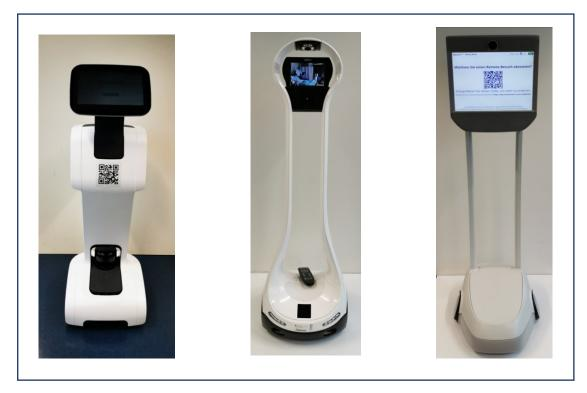
Figure 24: Different telepresence systems: TEMI (Temi Global Ltd.), VGo (Vecna Technologies) and BEAM (Blue Ocean Robotics) (Pictures: K. Türkogullari, Frankfurt UAS)
