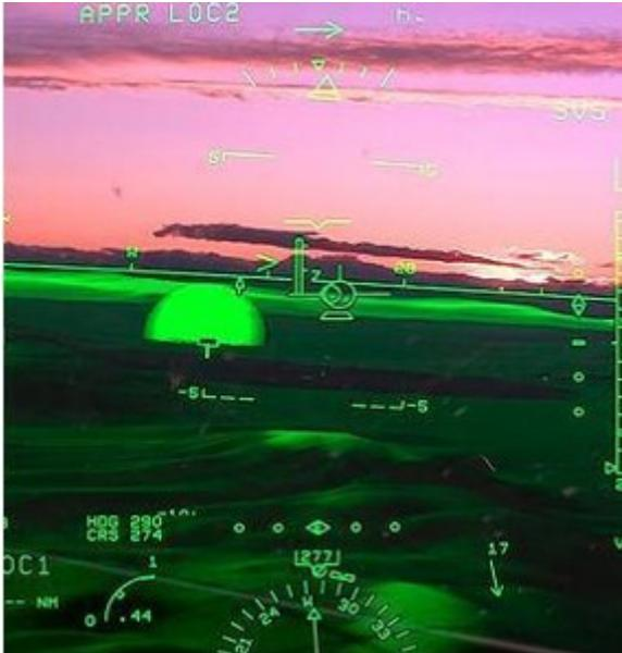
Figure 60: NASA's AR navigation system
