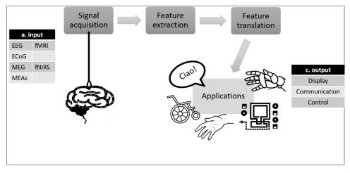
Figure 69: Functional blocks of a BCI system
