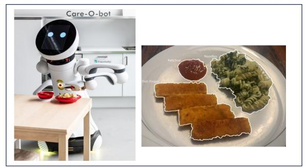
Figure 29: The Care-O-Bot 4 is able to identify food on a plate, to pick it up with a spoon and to present it in front of a person's mouth (Picture: R. Bez © Fraunhofer
