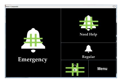
*Figure 74: An example of a user interface for a P300-based BCI. Green grid stimuli are overlapped to items on the screen.*
